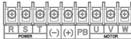
Figure 3-8 : 3PH Bornes du circuit principal (45-110 kW)
